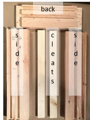
Sides and Back: Constructed from 2x6 lumber that has been milled with a dado grooves and rabbets. The upper groove is cut below the top to provide a permanent 3/8" hive opening. The upper dado groove is cut deep and wide enough to accept the drawer panel. The second dado groove holds a cleat used to support the length of the aluminum tray. The rabbets on the ends of the back piece will fully hide the grooves from the outside.
